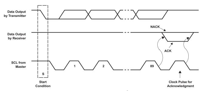
Figure 17. Acknowledgment on I<sup>2</sup>C Bus
