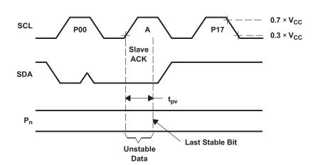
Write-Mode Timing  $(R/\overline{W} = 0)$
