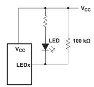
Figure 21. High-Value Resistor in Parallel With LED
