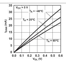
Figure 5. I/O Sink Current vs Output Low Voltage
