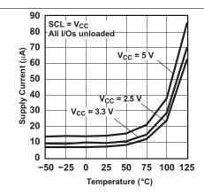
Figure 1. Supply Current vs Temperature
