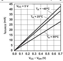
Figure 9. I/O Source Current vs Output High Voltage
