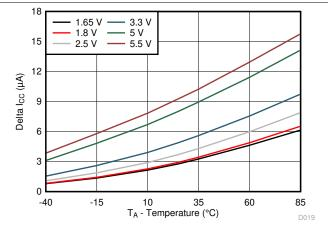
Figure 7-18.  $\Delta$  I<sub>CC</sub> vs Temperature for Different V<sub>CC</sub> (V<sub>I</sub> = V<sub>CC</sub> – 0.6 V)
