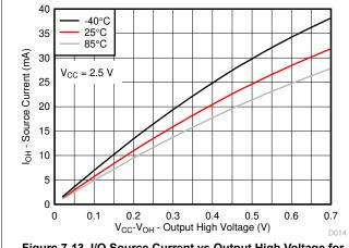
Figure 7-13. I/O Source Current vs Output High Voltage for Different Temperature (T<sub>A</sub>) for V<sub>CC</sub> = 2.5 V
