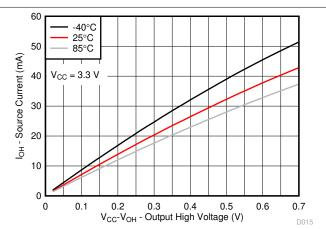
Figure 7-14. I/O Source Current vs Output High Voltage for Different Temperature (T<sub>A</sub>) for V<sub>CC</sub> = 3.3 V
