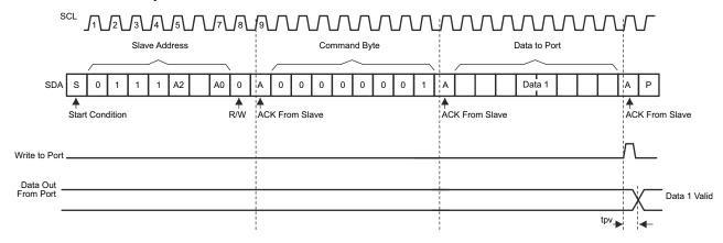
Figure 9-8. Write To Output Port Register
