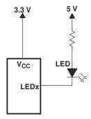
Figure 10-3. Device Supplied By A Lower Voltage
