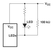
Figure 10-2. High-Value Resistor In Parallel With The Led
