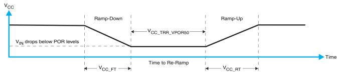
Figure 11-2. V<sub>CC</sub> Is Lowered Below The Por Threshold, Then Ramped Back Up To V<sub>CC</sub>
