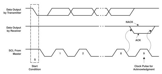
Figure 9-5. Acknowledgment On I<sup>2</sup>C Bus
