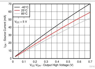
Figure 7-15. I/O Source Current vs Output High Voltage for Different Temperature ( $T_A$ ) for  $V_{CC}$  = 5 V
