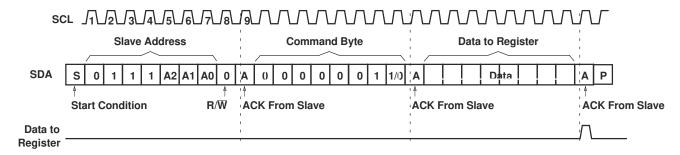
Figure 9-9. Write To Configuration Or Polarity Inversion Registers
