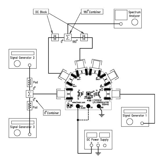
Figure 1. Proper Measurement Equipment Setup
