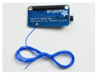
Hook the exposed wire end into the ANT hole
