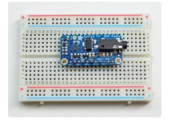
You're done! Check your solder joints visually and continue onto the antenna
