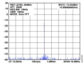
Figure 3. EV1HMC8342LS6 OUT (J4) Isolation, Input Frequency = 15 GHz, Input Power = 5 dBm,  $V_{GG2} = -0.8 V$ ,  $V_{GG1} = -1.25 V$ , Includes Insertion Loss of the RF Cable
