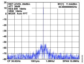
Figure 2. EV1HMC8342LS6 OUT (J4) RF Output, Input Frequency = 15 GHz, Input Power = 5 dBm, V<sub>GG2</sub> = -0.8 V, V<sub>GG1</sub> = -1.25 V, Includes Insertion Loss of the RF Cable
