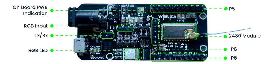
Most of the I/O pins on the module are broken out to the pin headers on sides of this board for easy interfacing, so users can easily connect peripherals with jumper wires.
