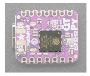
The ESP32-S2 is a highly-integrated, lowpower, 2.4 GHz Wi-Fi System-on-Chip (SoC) solution that now has built-in native USB as well as some other interesting new technologies like Time of Flight distance measurements. With its state-of-the-art power and RF performance, this SoC is an ideal choice for a wide variety of application scenarios relating to the Internet of Things (IoT) (https://adafru.it/ Bwq), wearable electronics (https:// adafru.it/Osb), and smart homes.
