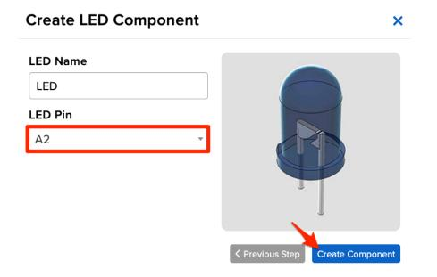
Adafruit IO will send a command to your board (running WipperSnapper) telling it to configure the GPIO pin as a digital output. Your QT Py device interface displays the new LED component.
