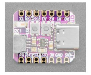
There are eleven GPIO pins broken out to pads. There is hardware I2C, UART, and SPI.
