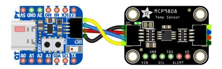
Note we are using the STEMMA QT port here, that means we need to reference Wire1 for I2C communication and also add Wire1.setPins(SDA1, SCL1) in our code in setup()
