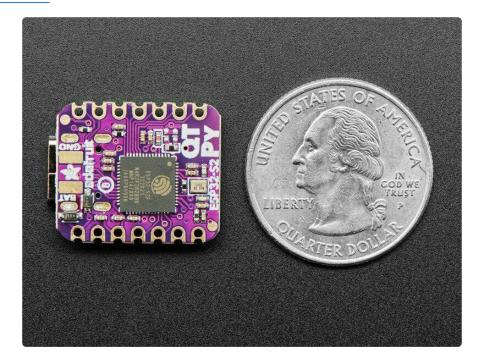
Please note the QT Py ESP32-S2 has a single-core 240 MHz chip, so it won't be as fast as ESP32's with dual-core. Also, there is no Bluetooth support. However, we are super excited about the ESP32-S2's native USB which unlocks a lot of capabilities for advanced interfacing! This ESP32-S2 mini-module we are using on the QT Py comes with 4 MB flash and 2 MB PSRAM so you can buffer massive JSON files for parsing!
