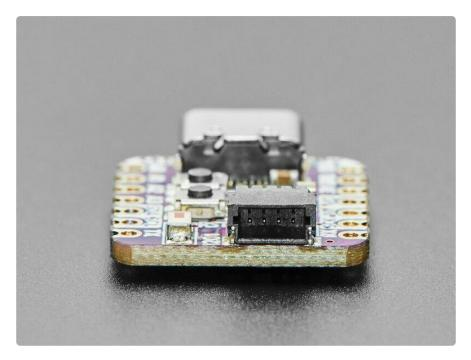
Pinout and shape are <u>Seeed Xiao</u> (https://adafru.it/NC3) compatible, with castellated pads. In addition to the QT connector, we also added an RGB NeoPixel (with controllable power pin to allow for ultra-low-power usage), a reset button (great for restarting your program or entering the bootloader) and a button on GPIO 0 for entering the ROM bootloader or for user input
