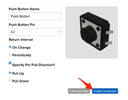
Adafruit IO should send a command to your board (running WipperSnapper), telling it to configure the GPIO pin you selected to behave as a digital input pin and to enable it to pull up the internal resistor.
