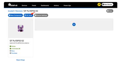
You should see a new pop-up showing a list of the I2C addresses detected by an I2C scan. If wired correctly, the AHT20's default I2C address of  $0\times38$  appear in the I2C scan list.
