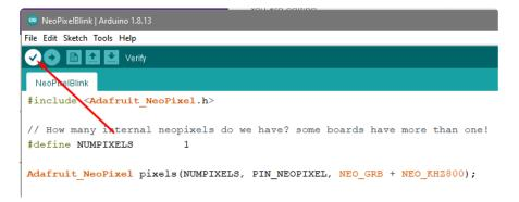
During verification/compilation, the computer will do a bunch of work to collect all the libraries and code and the results will appear in the bottom window of the IDE.
