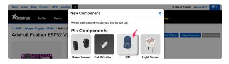
The QT Py contains GPIO pins that can be configured either as an input or an output. The "Create LED Component" screen tells Adafruit IO to configure a general-purpose output pin connected to the LED on your QT Py as a digital output so you can turn the LED on or off.
