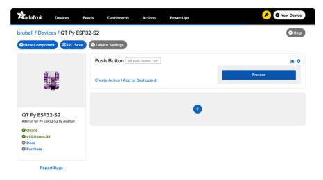
Press the button to change the value of the push button component on Adafruit IO.
