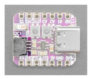
This JST SH 4-pin STEMMA QT (https:// adafru.it/Ft4) connector breaks out a second I2C interface (SCL1, SDA1, 3.3V, GND). It allows you to connect to various breakouts and sensors with STEMMA QT connectors (https://adafru.it/Qgf) or to other things using assorted associated accessories (https://adafru.it/Ft6). It works great with any STEMMA QT or Qwiic sensor/device. You can also use it with Grove I2C devices thanks to this handy cable (https://adafru.it/Ndk).
