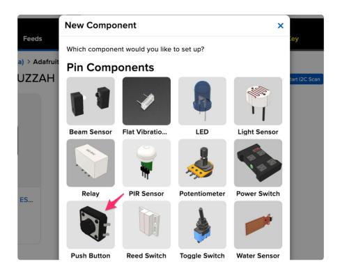
The next screen presents you with options for configuring the push button. Start by selecting the QT Py's digital pin you connected to the push button.
