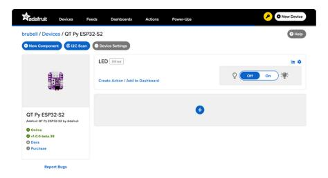
On the device interface, toggle the LED component by clicking the toggle switch. This should toggle the LED connected to your QT Py on or off.
