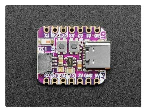
The ESP32-S2 is a highly-integrated, low-power, 2.4 GHz Wi-Fi System-on-Chip (SoC) solution that now has built-in native USB as well as some other interesting new
