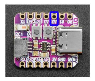
A2 (highlighted in blue) is the first pin used for capacitive touch.
