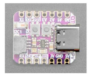
USB-C port - This is used for both powering and programming the board. You can power it with any USB C cable.
