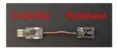
The I2C, or <u>inter-integrated circuit</u> (https://adafru.it/u2a), is a 2-wire protocol for communicating with simple sensors and devices, which means it uses two connections, or wires, for transmitting and receiving data. One connection is a clock, called SCL. The other is the data line, called SDA. Each pair of clock and data pins are referred to as a bus.
