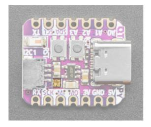
Above the SCK and MI on the silk, is the RGB NeoPixel LED. This addressable LED works both as a status LED (in CircuitPython and the bootloader), and can be controlled with code. It is available in CircuitPython as board.NEOPIXEL, and in Arduino as PIN\_NEOPIXEL. There is a NeoPixel power pin that needs to be pulled high for the NeoPixel to work. This is so it can be fully de-powered for low power usage. It is available in CircuitPython and Arduino as NEOPIXEL\_POWER.
