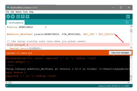
Turning on detailed compilation warnings and output can be very helpful sometimes - Its in Preferences under "Show Verbose Output During:" and check the Compilation button. If you ever need to get help from others, be sure to do this and then provide all the text that is output. It can assist in nailing down what happened!
