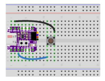
Make the following connections between the QT-PY and the button:
