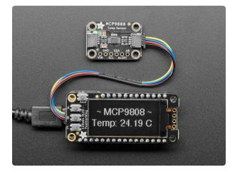
Adafruit MCP9808 High Accuracy I2C Temperature Sensor Breakout
