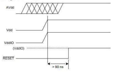
Note: When using external RESET at power-up, VddIO must not be enabled after Vdd
