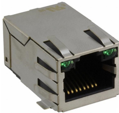
Figure 24: Ethernet PHY Status LEDs
