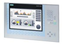
SIMATIC HMI KP1200 Comfort, Comfort Panel, key operation, 12" widescreen TFT display, 16 million colors, PROFINET interface, MPI/PROFIBUS DP interface, 12 MB configuration memory, Windows CE 6.0, (Microsoft Support included Security updates discontinued) configurable from WinCC Comfort V11
