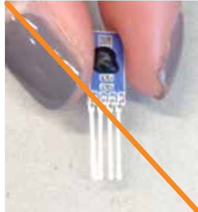
Sensor held with fingers without gloves
