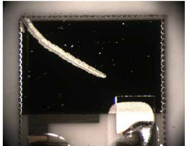
Picture 8: Sensor with a scratch
