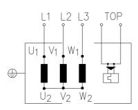
Change of rotation direction by reversing two phases
