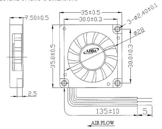
LEAD WIRES: UL 1571, AWG28, L=135+/-10 MM Red = positive; Black = negative.
