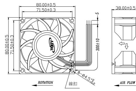
LEAD WIRES : UL 1061, AWG24 , L = 300±10 mm Red = positive ; Black = negative. White = FG ; Blue = pwm input
