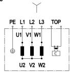
Note: Change of rotation direction by reversing two phases
