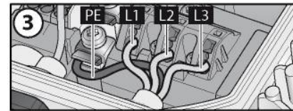
Fig. 2: Connecting wires to terminals
