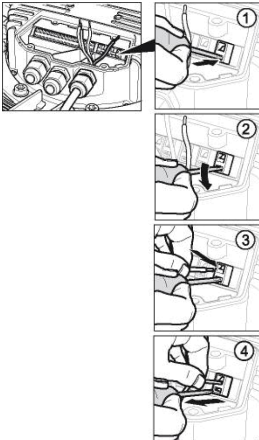
Fig. 2: Connecting the wires to terminals
