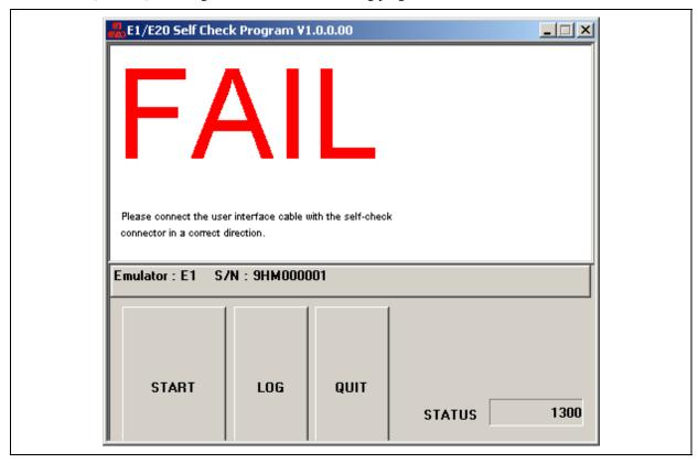
Figure A.4 [FAIL] at the Start of Self-Checking (without the Cable Connected to the Self-Checking Connector)
