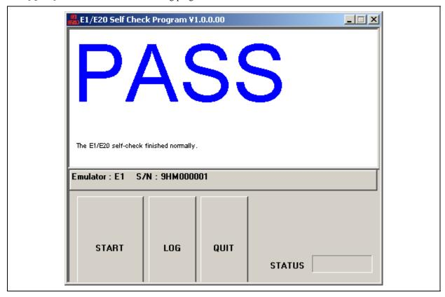
Figure A.10 Normal Completion of Self-Checking
