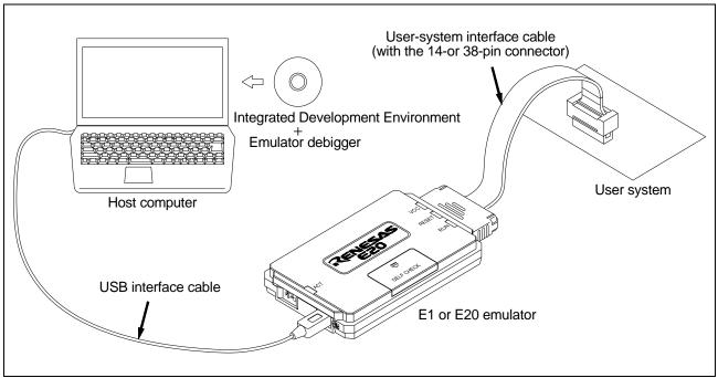
Figure 1.1 System configuration with an Emulator
