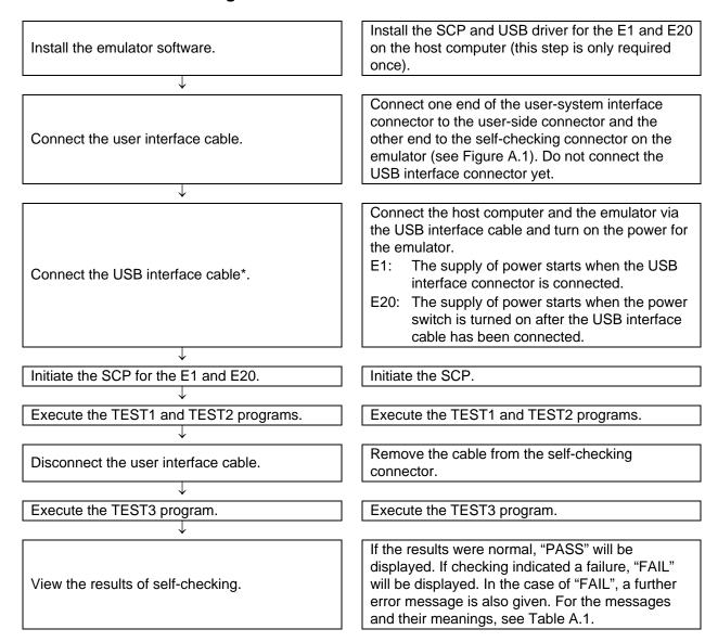
Note: Fault analysis of the hardware by using the self-checking program only works correctly when a single emulator is connected to the host computer. When two or more emulators are connected, correct operation is not guaranteed.
