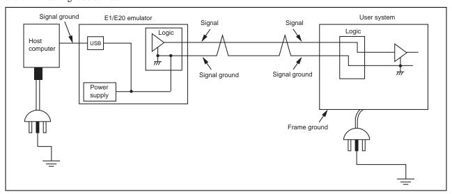
Figure 2.6 Connecting System Ground
