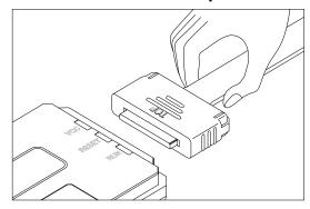
(1) A connector to the user-system interface cable must be installed on the user system. Table 2.1 shows the recommended connector for the emulator.
