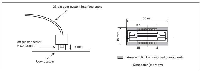
Figure 2.5 Connecting the User-System Interface Cable to the User System when the 38-Pin Connector is in Use with the E20
