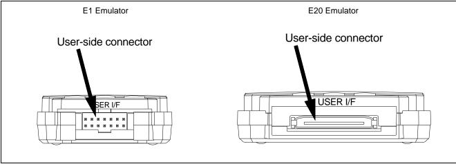
Figure 2.2 User-Side Connector on the E1 and E20
