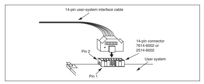
Figure 2.3 Connecting the User-System Interface Cable to the User System when the 14-Pin Connector is in Use with the E1
