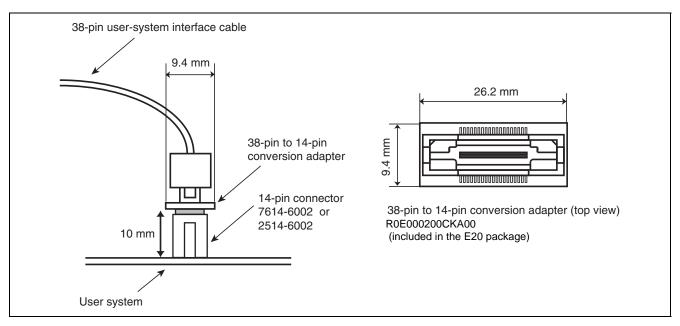
Figure 2.4 Connecting the User-System Interface Cable to the User System when the 14-Pin Connector is in Use with the E20
