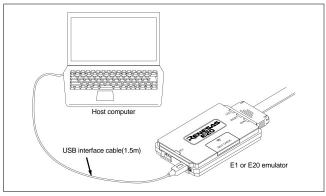
Figure 2.1 System Configuration when Connecting the Emulator to the Host Computer
