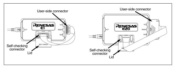
Figure A.1 Connecting the User Interface Cable (for the E1 and E20)
