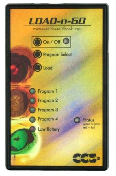
LOAD-n-GO is a hand-held mobile programmer and goes where no PC or laptop has gone before. This device allows for quick field programming of targets with up to four firmware images. The programming process is as easy as 1-2-3 with the LOAD-n-GO. Simply load the program into the LOAD-n-GO via a USB cable, connect to the target and program! LOAD-n-GO debug support covers all targets that have debug mode when used in conjunction with the C-Aware IDE Compilers.
