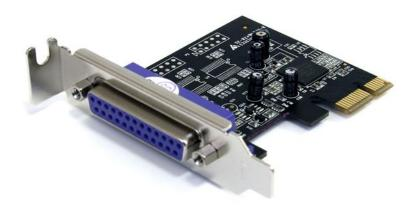
The PEX1PLP PCIe Parallel Adapter card can be installed in a PCI Express (PCIe) x1 slot, allowing you to connect EPP/ECP parallel peripherals to any computer, while relying on a native, single-chip design (Oxford OXPCIe952) that harnesses the capability of true PCI Express - ensuring maximum performance and reliability.
