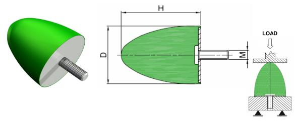
The Type VP Bobbin Mount End Stops are designed to be used on a wide range of applications to prevent shocks and over-loading thanks to their progressive absorption.
