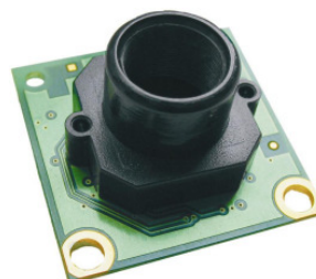
-M12 = camera with lens holder for M12 / 0.5 lenses (S-Mount)
