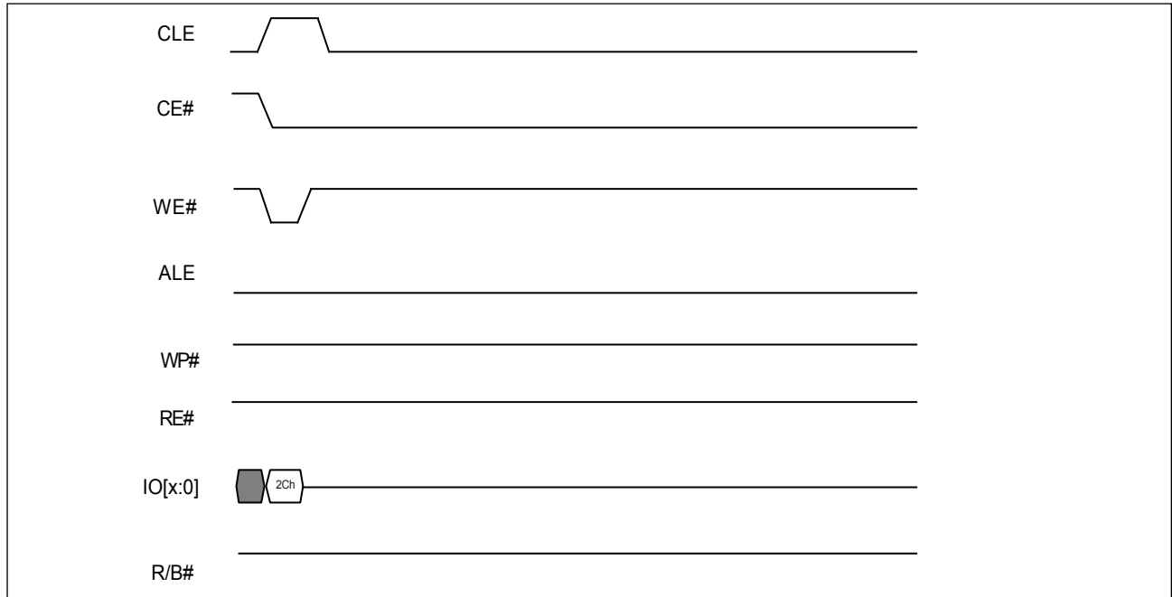
Figure 40. AC Waveforms for Block Solid-Protect
