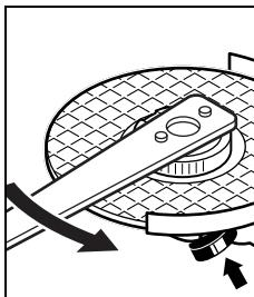
A properly attached, undamaged quick-clamping nut can be loosened by hand when turning the knurled ring in anti-clockwise direction. **Never loosen a tight quick-clamping nut with pliers. Always use the two-pin spanner.** Insert the two-pin spanner as shown in the illustration.
