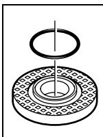
An O-ring (plastic part) is inserted in the mounting flange **8** around the centring collar. If the O-ring is missing or is damaged, it must in all cases be replaced (article number 1 600 210 039) before the mounting flange **8** is mounted.
