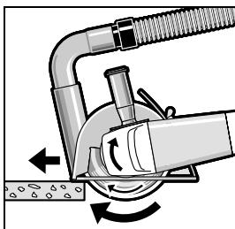
Switch on the machine and place the front part of the cutting guide on the workpiece. Slide the machine with moderate feed, adapted to the material to be worked.
