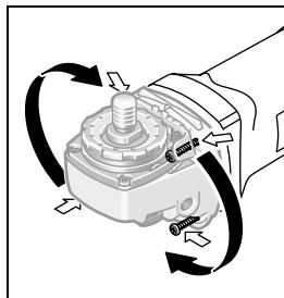
The machine head can be rotated with respect to the machine housing in 90° steps. In this manner, the On/Off switch can be brought into a more convenient position for special working situations,
