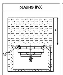
Continuous immersion in water IP68 test conditions
