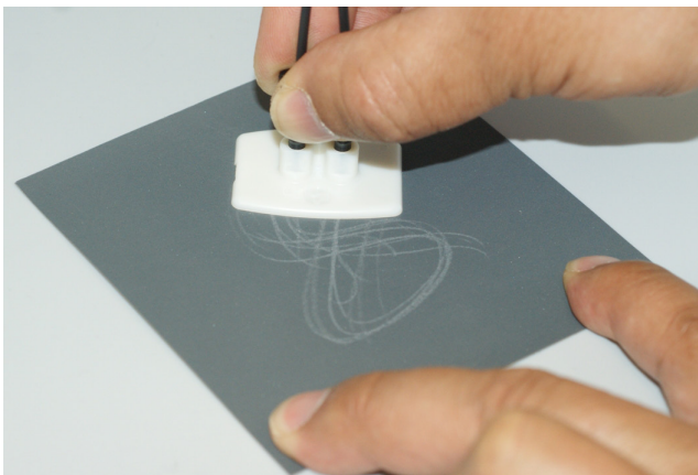
Figure 27. Polishing by drawing pattern 8 on abrasive paper
