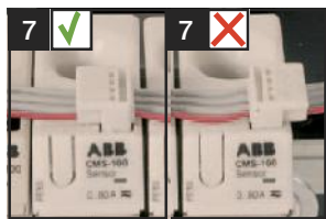
7 Plug the connectors to the sensors with the longer side to the middle
