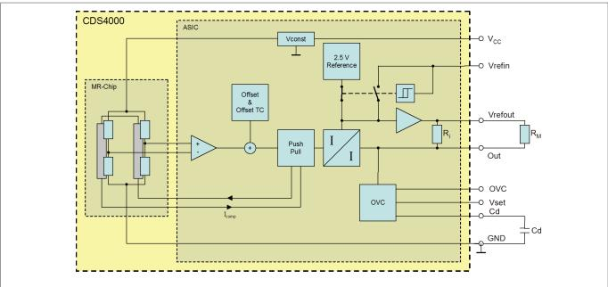
Fig. 1: Block diagram of CDS4000 current sensors.
