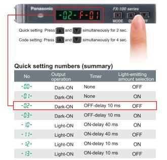
Refer to "Quick setting function" and "Code setting function" in "PRECAUTIONS FOR PROPER USE" for details.
