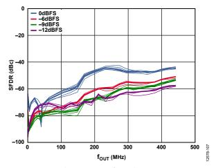
Figure 7. Single Tone SFDR vs. f<sub>OUT</sub> in the First Nyquist Zone over Digital Back Off, f<sub>DAC</sub> = 983 MHz
