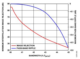
Figure 73. Interpolation Filter Performance Beyond Specified Bandwidth
