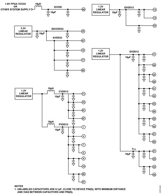
Figure 66. JESD204B Interface PCB Power Domain Recommendation
