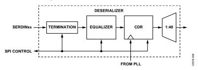
Figure 45. Deserializer Block Diagram
