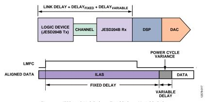
Figure 55. JESD204B Link Delay = Fixed Delay + Variable Delay
