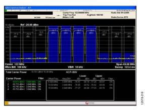
Figure 27. AD9136 Four-Carrier W-CDMA ACLR,  $f_{OUT}$  = 122 MHz,  $f_{DAC}$  = 983 MHz, 2× Interpolation, PLL Frequency = 122 MHz
