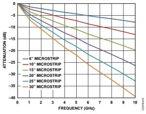
Figure 49. Insertion Loss of 50  $\Omega$  Microstrips on FR-4
