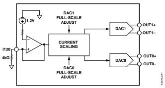
Figure 81. Simplified Block Diagram of DAC Core
