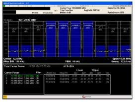
Figure 28. AD9135 Four-Carrier W-CDMA ACLR,  $f_{OUT}$  = 122 MHz,  $f_{DAC}$  = 983 MHz, 2× Interpolation, PLL Frequency = 122 MHz
