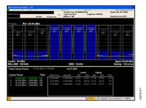
Figure 25. AD9136 Four-Carrier W-CDMA ACLR,  $f_{OUT} = 30$  MHz,  $f_{DAC} = 983$  MHz,  $2 \times$  Interpolation, PLL Frequency = 122 MHz
