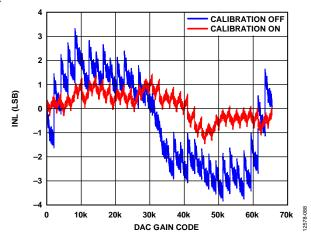
Figure 83. Precalibration and Postcalibration, INL
