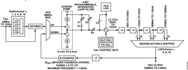
Figure 80. Device Clock PLL Block Diagram
