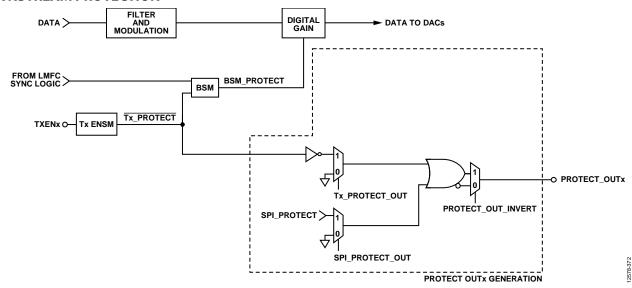
Figure 75. Downstream Protection Block Diagram
