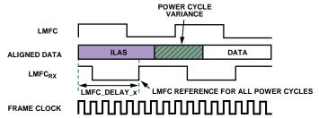
Figure 54. LMFC\_DELAY\_x, to Compensate for Link Delay > LMFC
