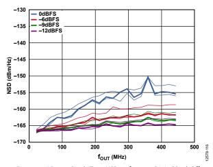
Figure 18. AD9136 Single Tone NSD vs.  $f_{\text{OUT}}$  over Digital Back Off,  $f_{\text{DAC}} = 983 \text{ MHz}$
