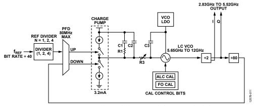
Figure 46. SERDES PLL Synthesizer Block Diagram Including VCO Divider Block
