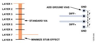
Figure 67. Minimizing Stub Effect and Adding Ground Vias for Differential Stripline Traces
