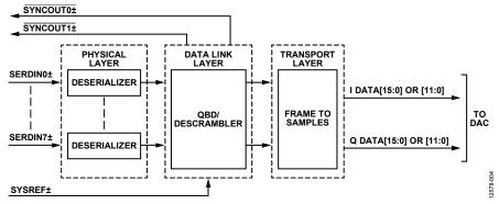
Figure 43. Functional Block Diagram of Serial Link Receiver
