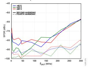
Figure 87. Postcalibration HD2 and HD4 over Temperature, Calibrated at 25  $^\circ\mathrm{C}$
