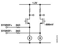
Figure 52. SYSREF± Input Circuit
