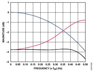
Figure 74. Responses of sin(x)/x Roll-Off, the Sinc-1 Filter, and the Composite of the Two-Input Signal and Protection
