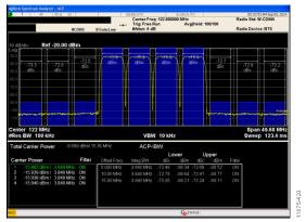
Figure 32. AD9135 Four-Carrier W-CDMA ACLR,  $f_{OUT}$  = 122 MHz,  $f_{DAC}$  = 1966 MHz, 4× Interpolation, PLL Frequency = 122 MHz
