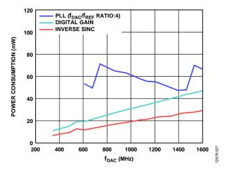
Figure 35. Power Consumption vs.  $f_{DAC}$  over Digital Functions
