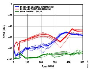
Figure 6. Single Tone Second and Third Harmonics and Maximum Digital Spur in the First Nyquist Zone, f<sub>DAC</sub> = 1966 MHz, 0 dB Back Off
