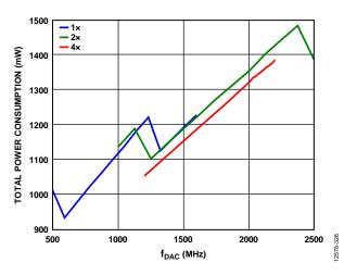
Figure 34. Total Power Consumption vs. f<sub>DAC</sub> over Interpolation, Eight SERDES Lanes Enabled, Digital Gain, Inverse Sinc and DAC PLL Disabled
