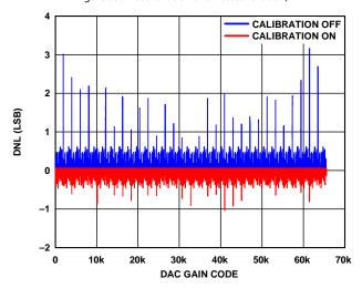
Figure 84. Precalibration and Postcalibration, DNL
