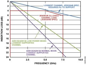
Figure 47. Insertion Loss Allowed
