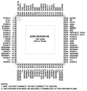
Figure 3. Pin Configuration
