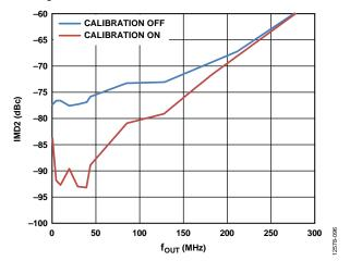
Figure 86. Precalibration and Postcalibration, IMD2
