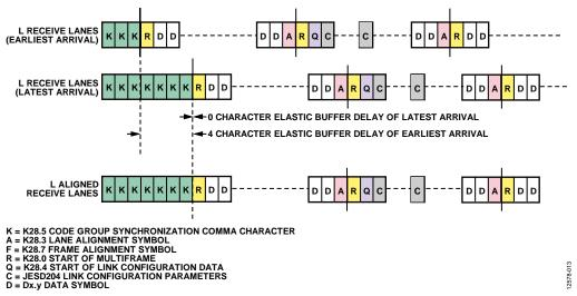
Figure 51. Lane Alignment During ILAS
