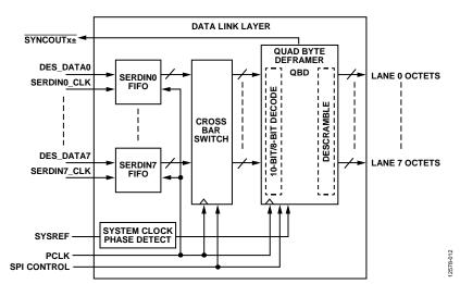
Figure 50. Data Link Layer Block Diagram
