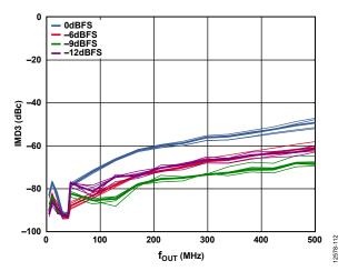
Figure 12. Two-Tone Third IMD (IMD3) vs.  $f_{OJT}$  over Digital Back Off,  $f_{DAC} = 1966$  MHz, Each Tone Is at -6 dBFS
