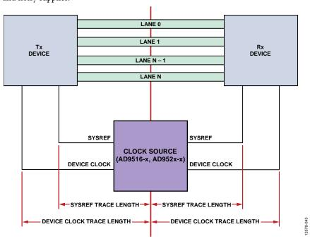
Figure 70. SYSREF Signal and Device Clock Trace Length
