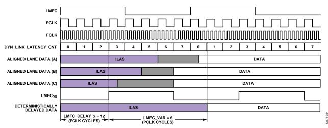
Figure 56. LMFC\_DELAY\_x Calculation Example
