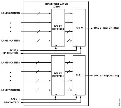
Figure 59. Transport Layer Block Diagram
