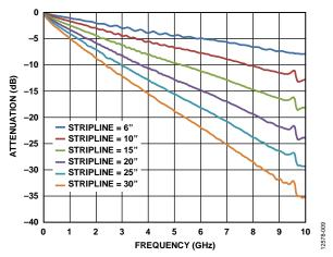
Figure 48. Insertion Loss of 50  $\Omega$  Striplines on FR-4
