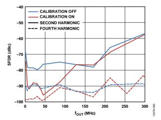
Figure 85. Precalibration and Postcalibration, HD2 and HD4
