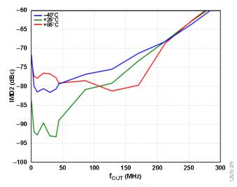
Figure 88. Postcalibration IMD2 over Temperature, Calibrated at 25°C
