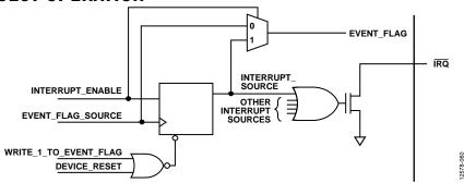
Figure 76. Simplified Schematic of IRQ Circuitry
