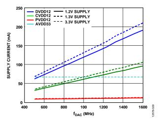
Figure 37. DVDD12, CVDD12, PVDD12, and AVDD33 Supply Currents vs. f<sub>DAC</sub> over Supply Voltage Setting
