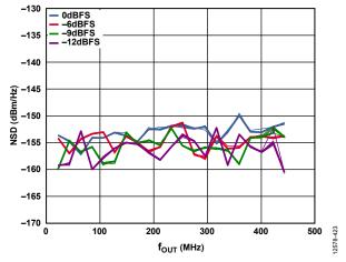
Figure 19. AD9135 Single Tone NSD vs.  $f_{OUT}$  over Digital Back Off,  $f_{DAC} = 983 \, \text{MHz}$
