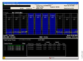
Figure 31. AD9136 Four-Carrier W-CDMA ACLR,  $f_{OUT}$  = 122 MHz,  $f_{DAC}$  = 1966 MHz, 4× Interpolation, PLL Frequency = 122 MHz
