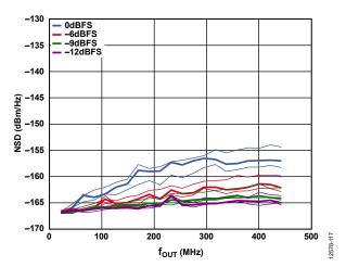
Figure 20. AD9136 Single Tone NSD vs.  $f_{OUT}$  over Digital Back Off,  $f_{DAC} = 1966 \, \text{MHz}$
