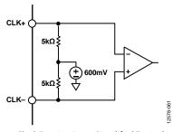
Figure 77. Clock Receiver Input Simplified Equivalent Circuit
