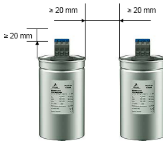
Figure 4: Minimum space over and between the capacitors.
