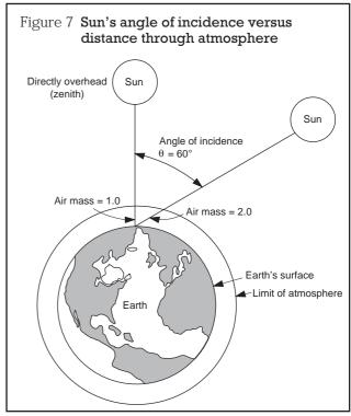
The value of air mass at any given time and location can be easily calculated using the relations shown on next page. The higher the value of air mass, the greater the attenuating effect of the atmosphere.
