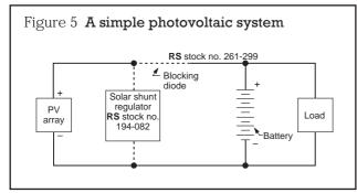
**Note:** The solar regulator includes a blocking diode and therefore a blocking diode should only be incorporated in a system when the solar regulator is not being used.
