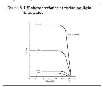
The graph above shows that there is no significant drop in cell voltage until insolation drops to 80W/m2.
