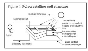
Cells are then tested and matched together with cells of similar performance for building up into series and parallel matrices to give the PV module the desired electrical characteristics.
