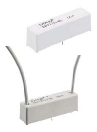
Very high isolation voltages - up to 15kV are achieved through the use of high vacuum reed switches with either rhodium or tungsten contacts which make these relays suitable for high reliability applications, such as cardiac defibrillators, test equipment and high voltage power supplies.
