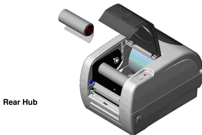
Fig. 5 Ribbon installation (II)
