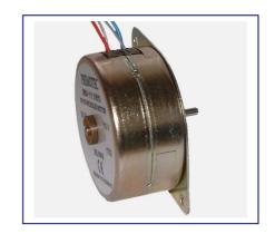
The windings of the 9904 111 31813 motor has been specifically designed for dual voltage operation, a 6.8K Ohm resistor used in series when operation from a 220 Vac supply is required.
