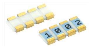
PRAHT arrays can be used in most applications requiring a matched pair (or set) of resistor elements at very high temperature up to 230 °C. The networks provide 2 ppm/°C TCR tracking, a ratio tolerance as tight as 0.05 % and outstanding stability.
