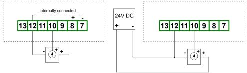
Figure 4.14. Connection of voltage converters
