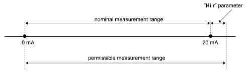
Figure 6.2. Definitions of measurement ranges in mode 0 ÷ 20mA
