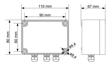
Figure 4.1. Device and assembly dimensions
