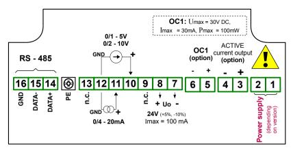
Figure 4.7. Terminals description (OC-type and active current outputs)
