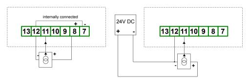
Figure 4.13. Connection of 3-wire current converters
