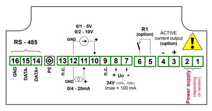
Figure 4.6. Terminals description (relay and active current outputs)
