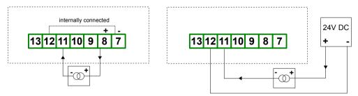
Figure 4.12. Connection of 2-wire current converters
