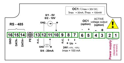
Figure 4.11. Terminals description (OC-type and active voltage outputs)
