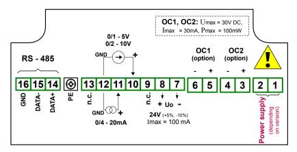
Figure 4.5. Terminals description (OC-type outputs)
