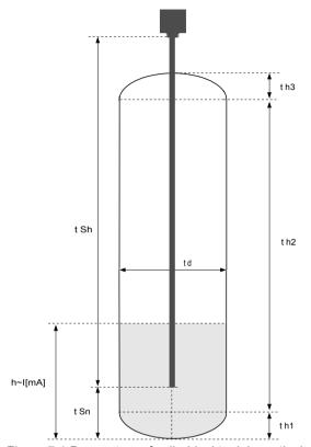
Figure 7.1 Parameters of cylindrical tank in vertical position.
