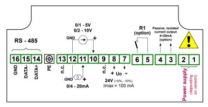
Figure 4.8. Terminals description (relay and passive current outputs)
