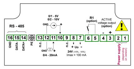
Figure 4.10. Terminals description (relay and active voltage outputs)
