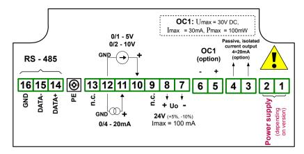
Figure 4.9. Terminals description (OC-type and passive current outputs)
