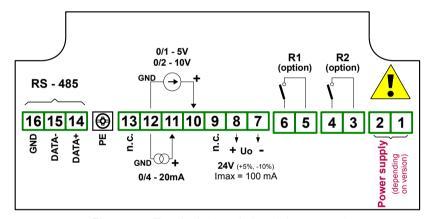
Figure 4.4. Terminals description (relay outputs)
