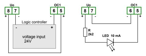
Figure 4.17. Example of OC-type outputs connection
