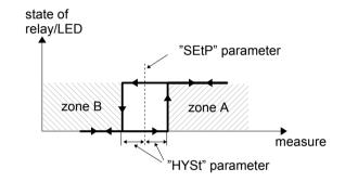
Figure 6.4. One threshold control of the relay/LED outputs
