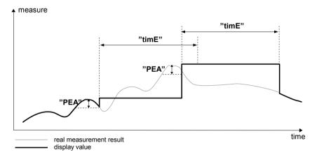
Figure 6.3. Process of peaks detection
