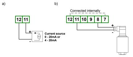
Figure 4.21. Connections of 2-wire sensor: a) active b) passive (needs additional supply)
