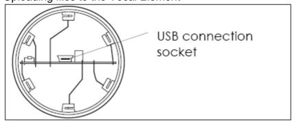
Connect the Vocal Element to one of the PC's USB sockets using the USB cable provided. The element appears as a removable medium in Windows Explorer.
