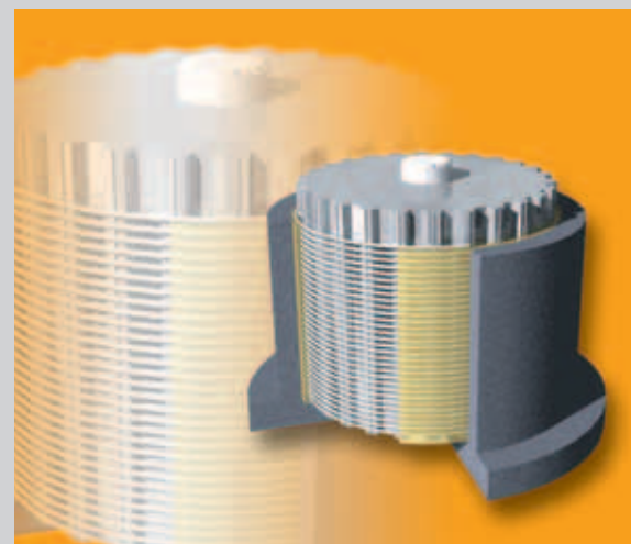
Casting mould, illustrated with a spirally wound tension member on the mould core
