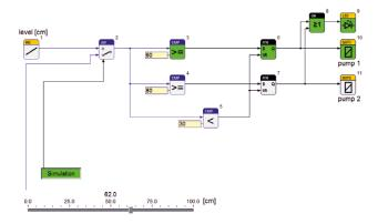
Programming the STG-600 follows using the USB port of your PC with installed miCon-L software suite.
