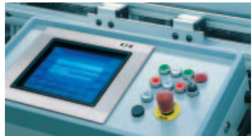
The touch panel visualizes the application and serves as the operator interface.
