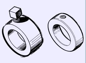
Set screw collars derive all their holding power from the screw as it is tightened onto the shaft. Holding power depends greatly on the shaft material and condition. For a set screw shaft collar to achieve maximum grip, the shaft must be of softer material than that of the set screw. This allows for impingement of the screw point into the shaft, which keeps the collar in its installed position under torque and axial loads, and prevents it from sliding along the shaft.
