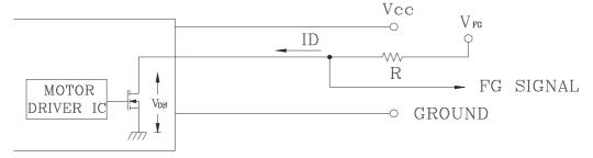
CAUTION: THE FG SIGNAL LEAD WIRE MUST BE KEPT AWAY FROM "+" LEAD WIRE & "-" LEAD WIRE.
