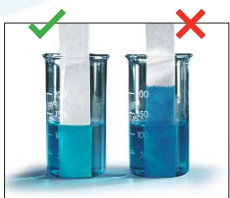
Filter media actively repels oil and water
