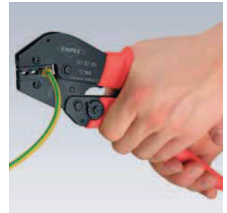
Third step: when greater hand force is required, such as e.g. when crimping insulated connectors 6 mm 2 , two-hand operation is possible by the longer handles
