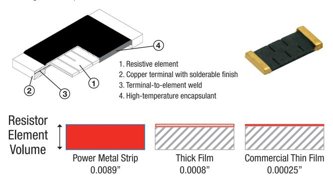
Power Metal Strip resistors are frequently used in applications that experience high-energy, short-term pulse transients:
