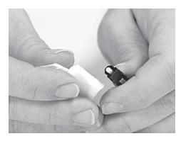
Note: Since the 3M™ Crimplok™ Connector is epoxyless, the mechanism that ensures fiber contact is different from epoxy connectors. The Crimplok connector and termination procedure are designed to produce a fiber protrusion of 15 to 40 microns. A slight protrusion is required to ensure contact at 140°F (60°C). Fiber protrusion will usually be noticed when cleaning the connector with a lint-free cloth. The product will interface with epoxyless and epoxy based connectors.
