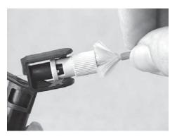
3.13 Hold the connector, and push the crimp ring into place until it seats.
