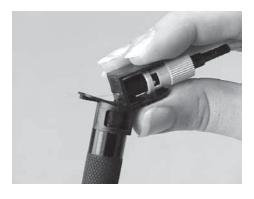
3.18 Press the connector forward to ensure that the ferrule is still seated against the stop.
