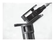
3.7 For SC only: While holding the aramid yarn and the activation tool in one hand, load the gold sleeve of the connector into the .120" cavity of the crimp tool. Partially close the crimp tool to secure the connector.
