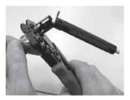
3.9 For ST: Cut the aramid yarn 1/2 to 5/8 inch from the end of the outer jacket.
