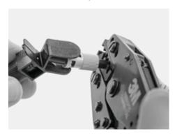
3.15 For buffered fiber, slide clear strain relief tube into crimp ring.
