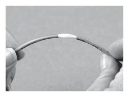
3.4 For SC: Strip fiber. Leave 3/8 to 1/2 inch (9 to 12 mm) of buffer protruding from jacket.
