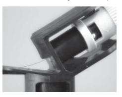
3.19 Add a two inch piece of Scotch® Magic Tape or Scotch® Transparent Tape to the top of the activation lever to catch cleaved fiber scrap.
