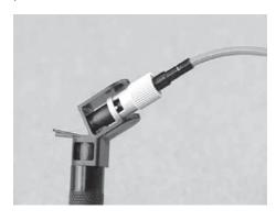
3.14 Crimp the large diameter section of the crimp ring with the .190" cavity of the crimp tool.
