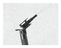
3.16 For SC: Crimp only the end of the smaller diameter of the crimp ring with the .137" cavity of the crimp tool to the 3 mm jacket. Do not crimp the middle portion of the crimp ring.
