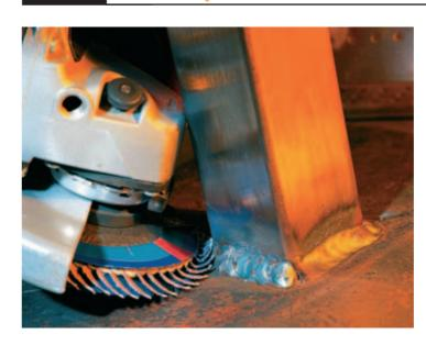
The Norton flexi-disc is a new concept in metal finishing which answers the customer demands for a more flexible disc with good stock removal.
