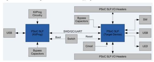
The PSoC 5LP Prototyping Kit is simplistic in design and focuses on providing you with complete access to develop applications using the PSoC 5LP device family. This kit supports the following features:
